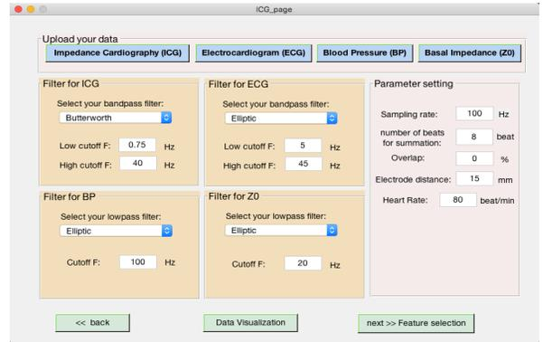
Fig. 6: Example of second page of GUI specialized for preprocessing of ICG signal.
